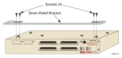
Figure 3-2 Attaching the Strain-Relief Bracket
